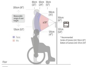
NOTE The iA1000 camera can be installed at a height which accommodates the user base.
